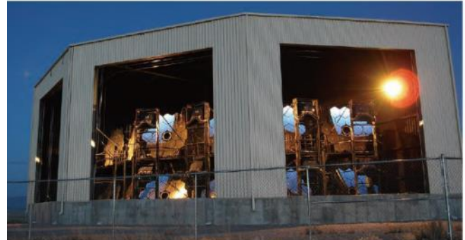
The fluorescence telescopes of The Telescope Array, the world's largest cosmic ray detector in the northern hemisphere. Fluorescence photons, a faint UV emission from air molecules, are detected when a cosmic ray strikes the atmosphere within the area of 700 km 2 around the telescopes.
