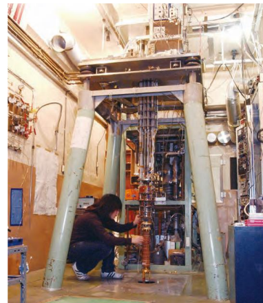
The Physics Department has a unique double-stage nuclear adiabatic demagnetization cryostat which is one of the very rare refrigerators in the world. It can achieve absolute temperatures below 0.01 mK and has been used to study superfluidity.
